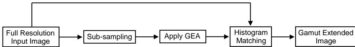
Figure 7. A schematic to reduce the computational cost of the proposed framework.
